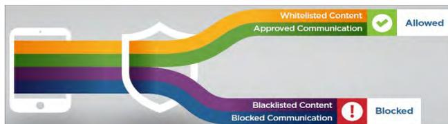
The network is protected by routers/firewalls that utilize a “default deny” approach to access controls utilizing whitelisted services / ports for our products and services. The GTL external network communication employs encrypted
