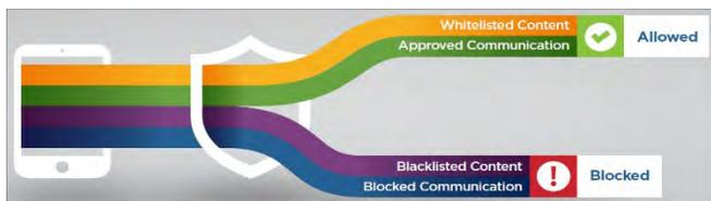
routes through a Gateway server appliance, which is both a firewall (to limit connections to a strict whitelist of allowed devices and allowed destination URLs) and a proxy server (to ensure no direct connection to the
