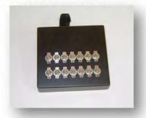
Mechanical cut-off switches may be provided as an alternative to phone shut down using the system workstation. These manual overrides or "kill switches" are used to quickly turn the telephones on/off on demand. Multi-phone kill switches will be installed at each control center or as specified by the facility.
